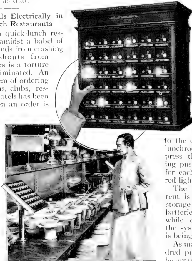
Press the "Pork and Beans" button and the "Pork and Beans" light flashes up in the kitchen. Thus you can now order your own meal in a certain Chicago lunchroom, or a waiter can order it noiselessly
